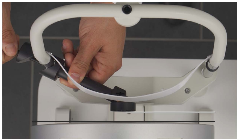
Fig. 21-4: Align the reference sphere in parallel (device as seen from above)
