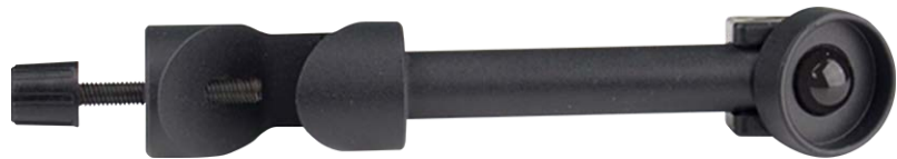
Fig. 21-3: Sphere holder with reference sphere
