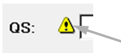
Fig. 14-5: Sign to perform maintenance
