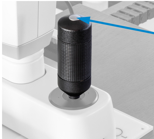
Fig. 8-1: Joystick with trigger button (arrow)
