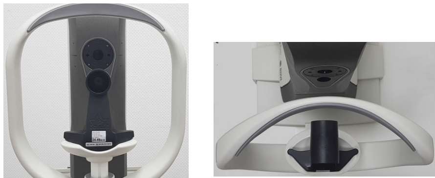
Fig. 14-1: Installation of the reference tool
