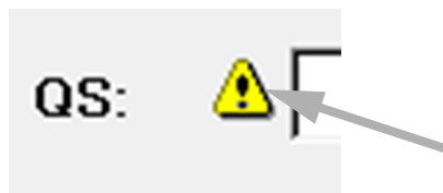
Fig. 14-5: Sign to perform maintenance
