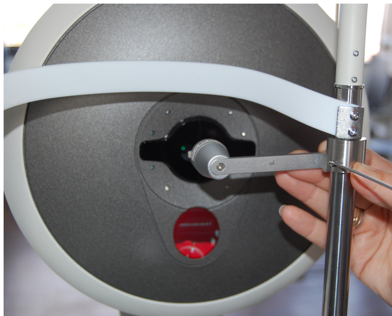
Fig. 10-1: Attach the test eye
