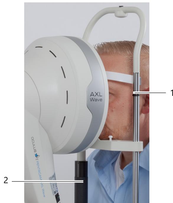
Fig. 8-1: Rough adjustment of the chin and forehead rest
