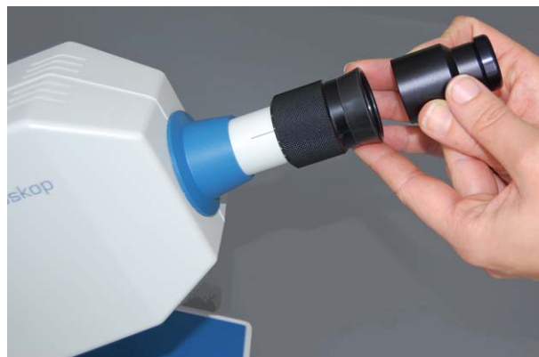
Fig. 8-1: Mounting the optical attachment lens.
