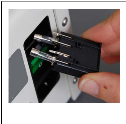
Fig. 12-3: Replacing the fuse
