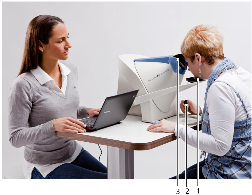
1 Chin rest (only Easyfield® C) 2 Manual button 3 Forehead rest Fig. 6-2: Application parts
