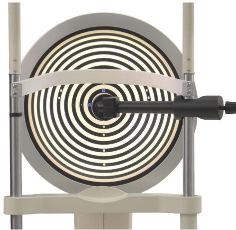
Fig. 15-4: Aligning the reference sphere height
