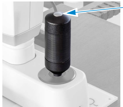
Fig. 3-2: Joystick with trigger (top)
