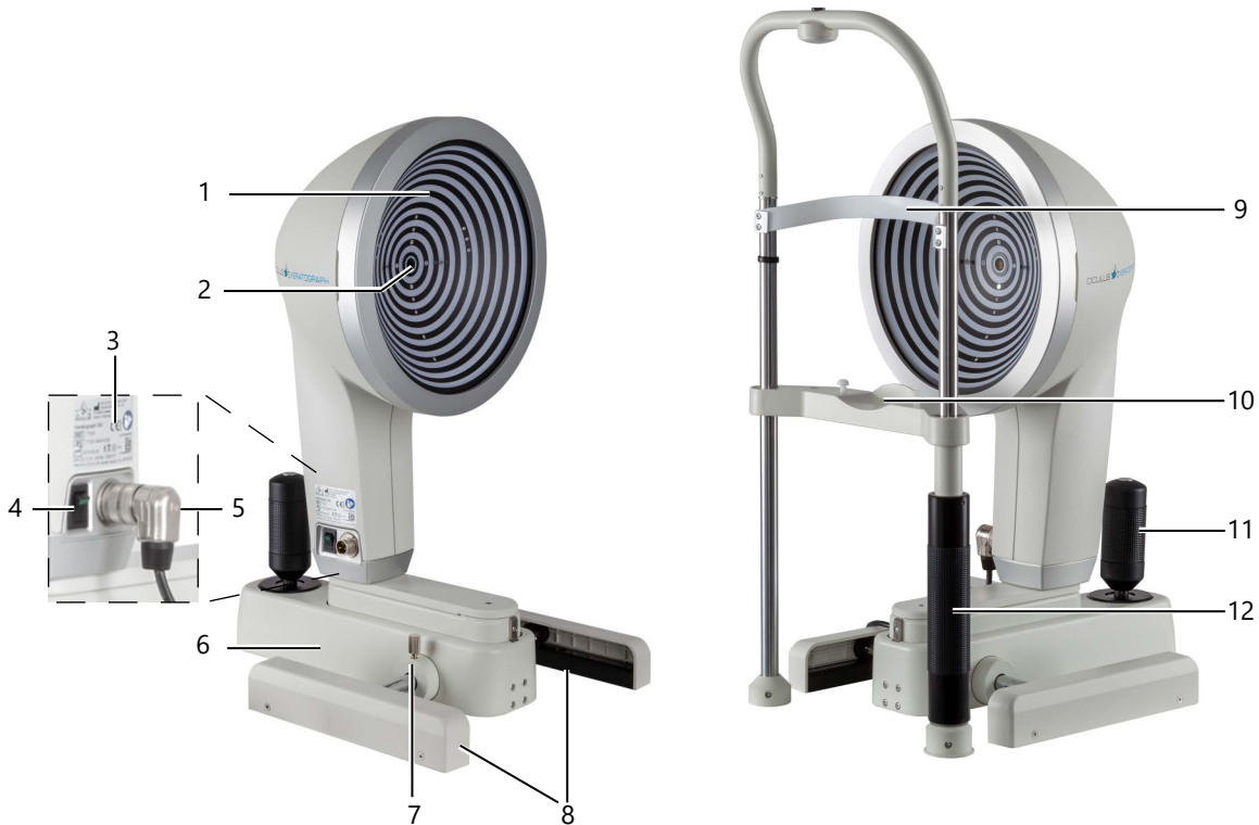
Fig. 3-1: K5 without chin/forehead rest (left) and with chin/forehead rest (right)
