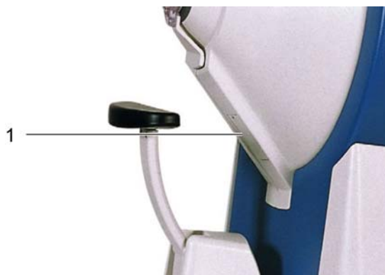
1 Cover of the background illumination bulb
