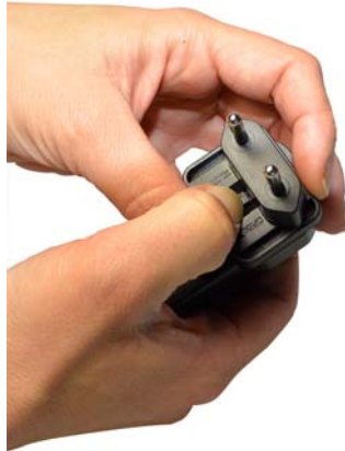
Fig. 7-4: Mounting an adapter corresponding to your country (example: power supply)
