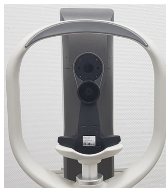
Fig. 10-1: Installed test eye
