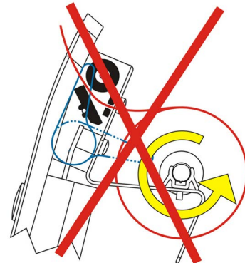
Fig. 11-5: Incorrect paper guidance
