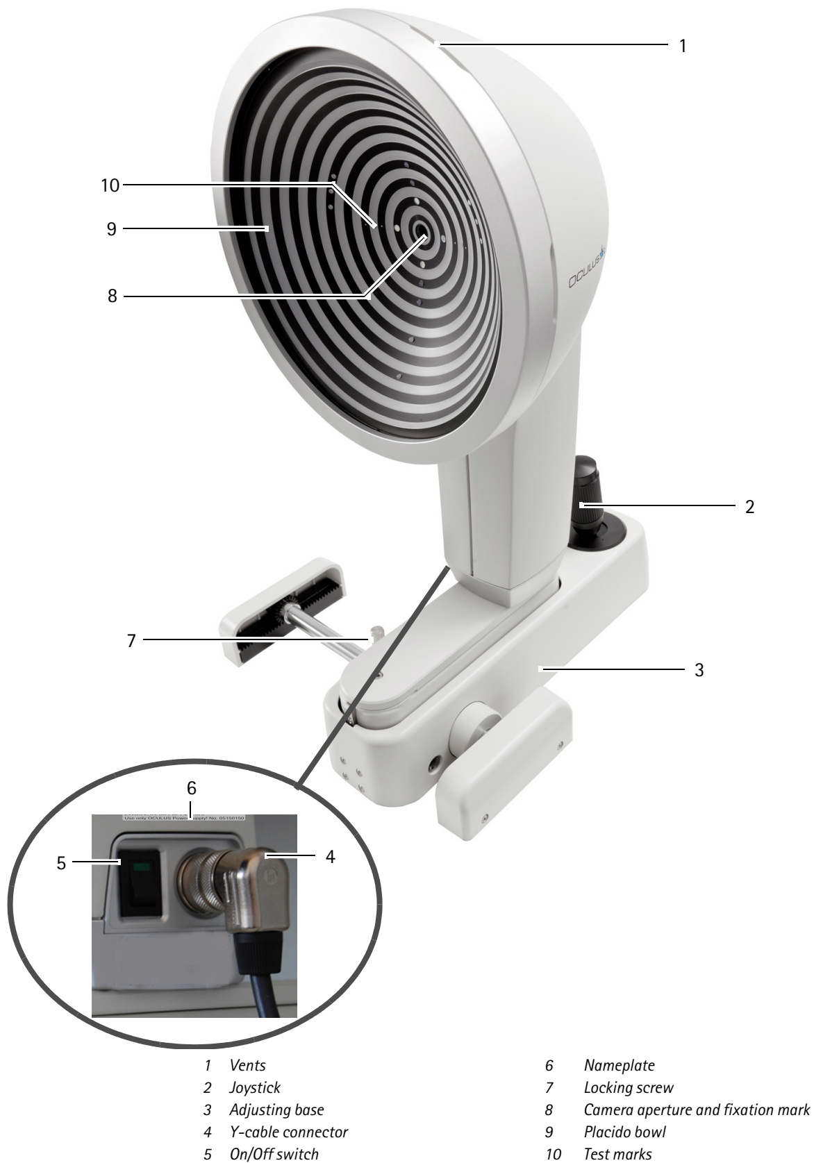
Fig. 6-1: Equipment overview of the Keratograph 5M
