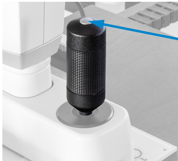
Fig. 8-1: Joystick with trigger button (arrow)
