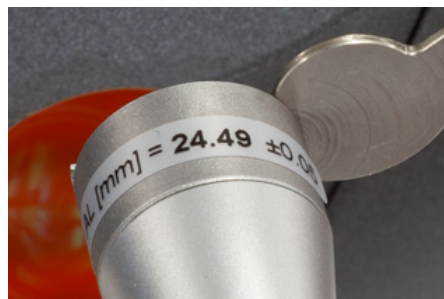
Fig. 9-4: Axial Length Test Eye
