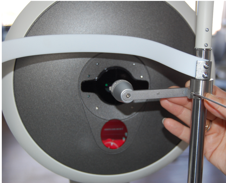
Fig. 9-1: Attach the test eye
