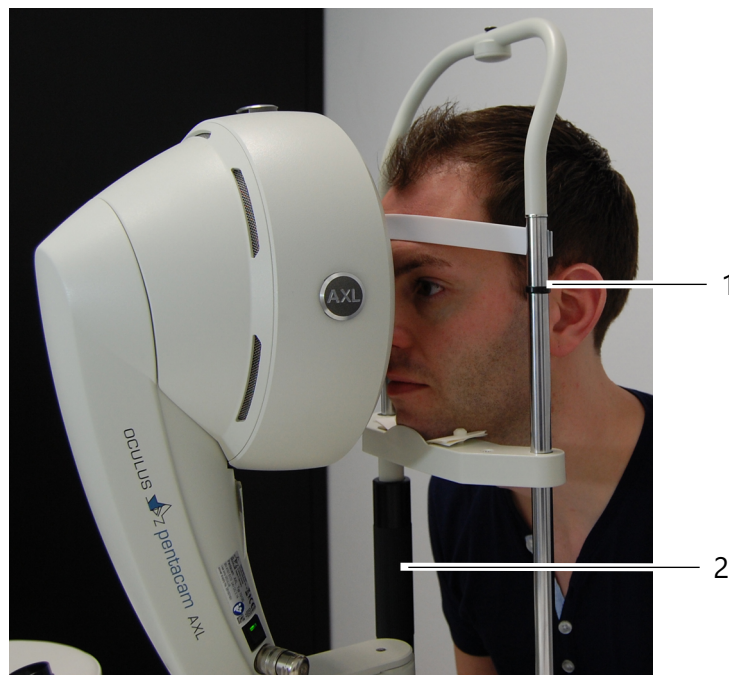
Fig. 7-8: Rough adjustment of the chin and forehead rest
