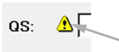
Fig. 14-5: Sign to perform maintenance
