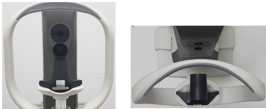
Fig. 14-1: Installation of the reference tool
