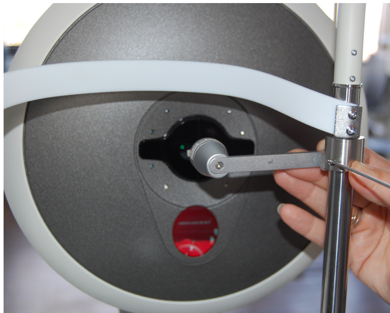
Fig. 13-1: Attach the test eye
