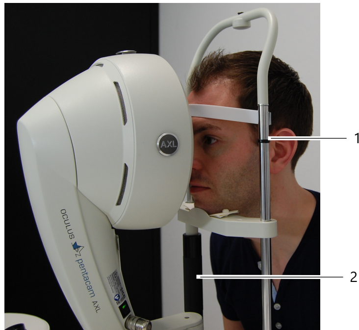
Fig. 7-2: Rough adjustment of the chin and forehead rest
