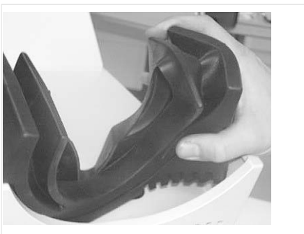
Fig. 13-3: Removing the viewer enclosure
