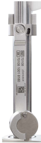
Fig. 13-2: Test eye in park/home position
