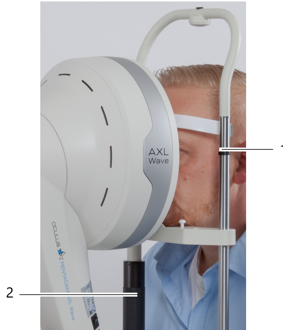
Fig. 11-1: Rough adjustment of the chin and forehead rest
