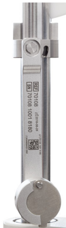
Abb. 13-2: Testauge in Parkposition
