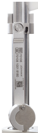
Abb. 13-2: Testauge in Parkposition
