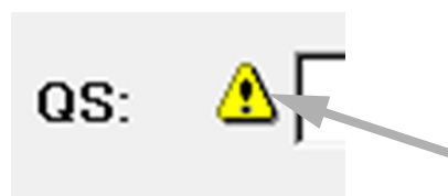
Fig. 14-5: Sign to perform maintenance
