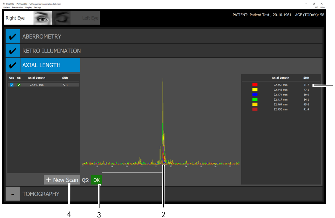
1 Single scans with SNR values 2 Signal to noise ratio of the axial length measurement 3 "QS" value 4 [+New Scan] button Fig. 11-14: Pentacam® AXL Wave program with "QS" display
