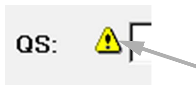
Fig. 14-5: Sign to perform maintenance
