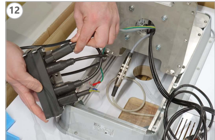
→ Connect power cable for lifting column
