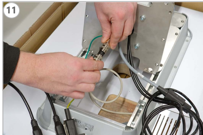
→ Connect the control cable for the lifting column.
